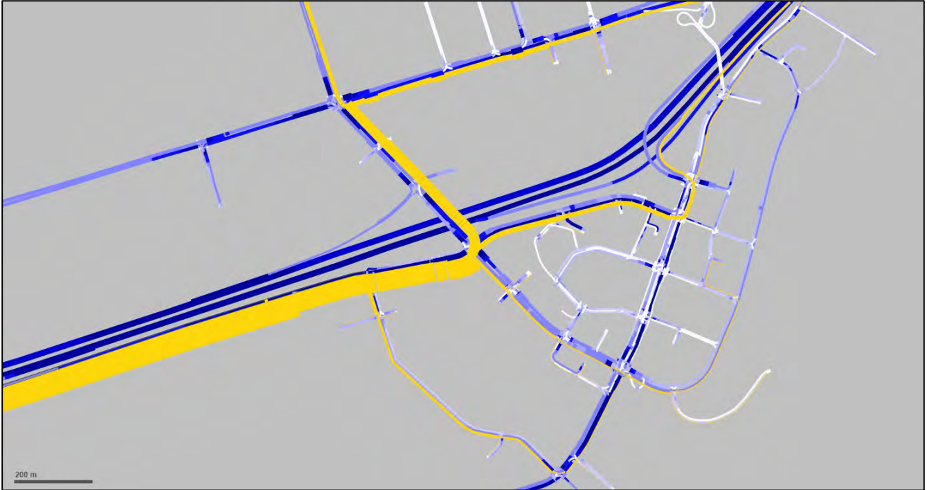
Figure 30: Alternative 2 (Additional Traffic Capacity) Off-Ramp Flow Bundles - Eastbound Direction during AM Peak Hour
