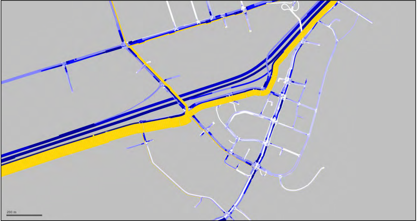
Figure 32: Alternative 3 (Additional Traffic Capacity, Modified Gardiner Ramps, New Lake Shore Ramp, Park Lawn at 2-Lanes) Off-Ramp Flow Bundles - Eastbound Direction during AM Peak Hour
