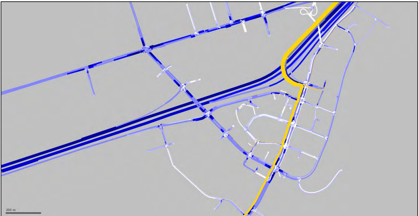
Figure 31: Alternative 2 (Additional Traffic Capacity) Off-Ramp Flow Bundles - Westbound Direction during PM Peak Hour
