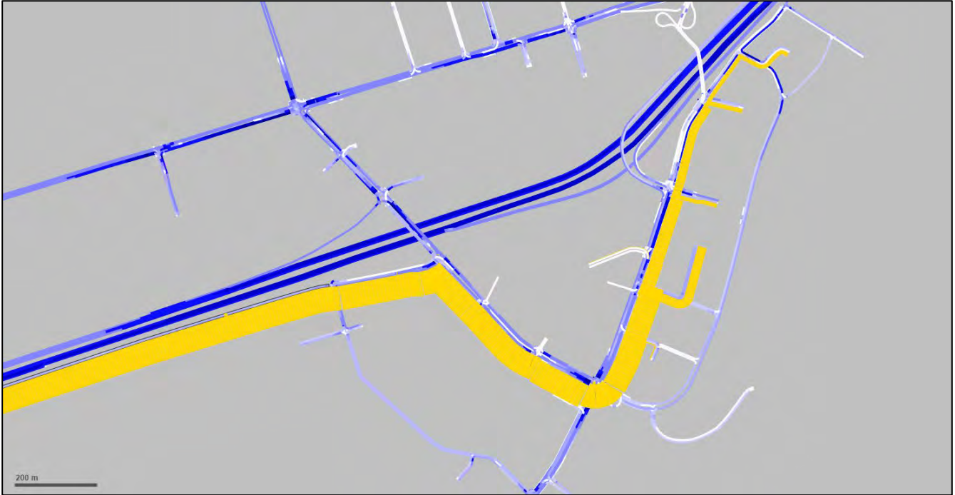
Figure 28: Alternative 1 (Future Do-Nothing) Off-Ramp Flow Bundles - Eastbound Direction during AM Peak Hour
