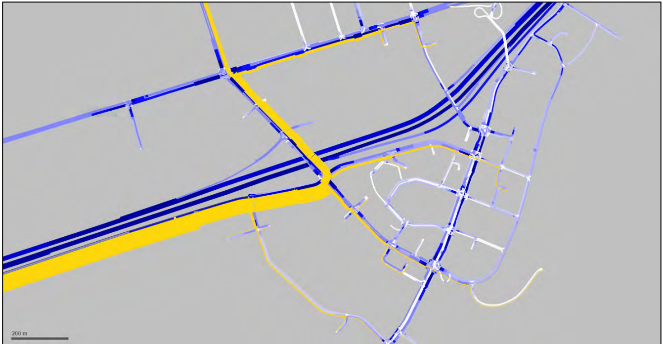
Figure 36: Alternative 4B (Neighbourhood Main Streets, 4-Lane Lake Shore) Off-Ramp Flow Bundles - Eastbound Direction during AM Peak Hour
