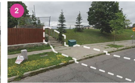
Potential raised crossing at Firgrove, with accessible ramp, and in-road traffic calming posts
