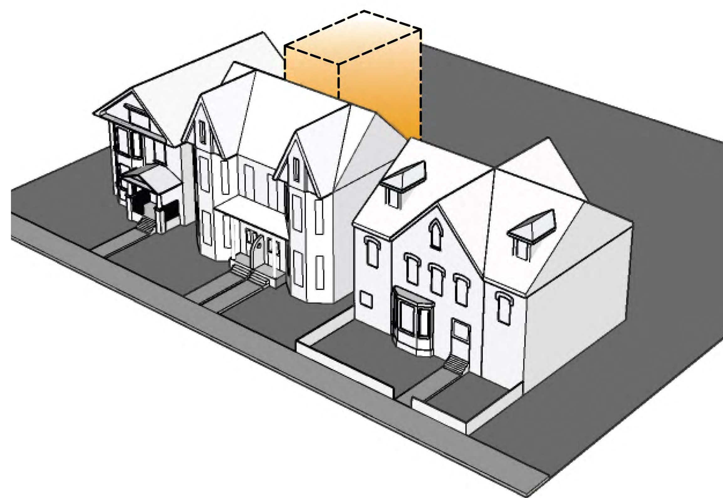
Concept Diagram | Schematic model illustrating a rear addition to a primary structure
