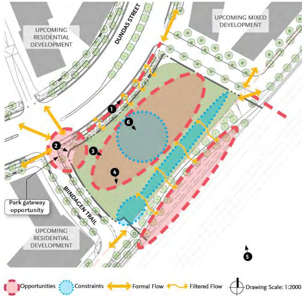
4 Constraint – Adjacency to rail tracks creates a higher noise condition at south edge, requiring screening / buffering of sound.
