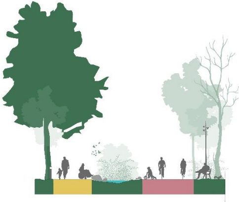
2.28 At times, the Green Spine's accessible path and bi-directional bike-way will be separated by planted green infrastructure features, as illustrated by this portion of the Green Path in Copenhagen.
