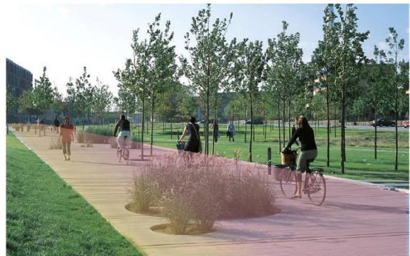
2.30 Portions of the Green Spine may encourage the mingling of different modes without compromising safety. The blending of cyclists and pedestrians at Nørrebroparken in Copenhagen, introduces design features that encourage slower, safer travel speeds.
