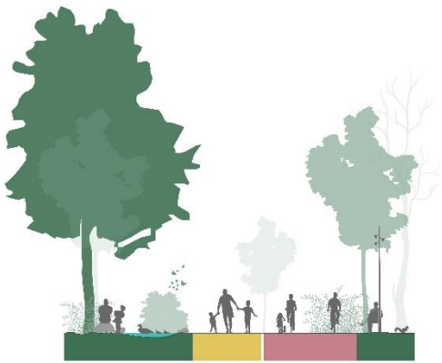
2.29 The Green Spine's pedestrian path and bi-directional bike-way may come together while maintaining the safety of pedestrians and cyclists, as shown along the Green Path in Copenhagen.
