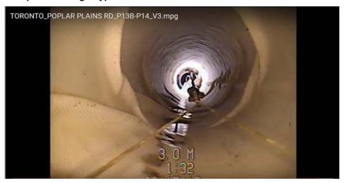
**Root Cause:** Helical fold due to the rotation of liner during insertion. This could also be influenced by swab movement during the forming stages.
