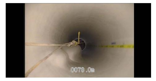
**Root Cause:** Multiple lumps due to external pressure (water or air) during the forming of the liner. **Description:** Large size ovoid lump with smaller sister lump along the bottom of the liner. Width at large lump base is 15%-25% of the circumference of the liner. Height of the lump is >30% of the diameter of the liner. Lump poses a problem to the liner by reducing hydraulic carrying capacity and providing a stress concentration point that can reduce the pressure class of the liner.
