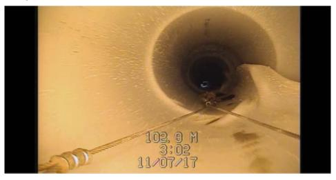
**Root Cause:** Large fold caused by the liner passing through a section of pipe with reduced diameter compared to the diameter of the host pipe the liner was sized for.
