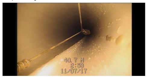
**Root Cause:** Standard fold due to slight over-sizing of the liner to ensure tight fit. **Description:** Thin and short longitudinal fold which runs the length of the installed liner.
