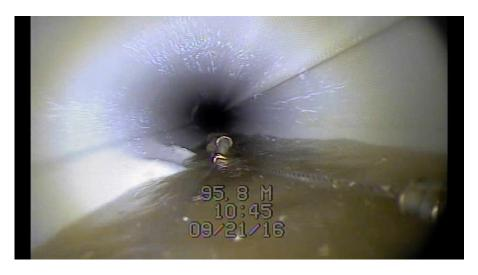
**Root Cause:** Lining over a foreign object such as a cork, swab piece, etc... This defect cannot have been caused by a substandard service as it is located on the bottom of the liner.
