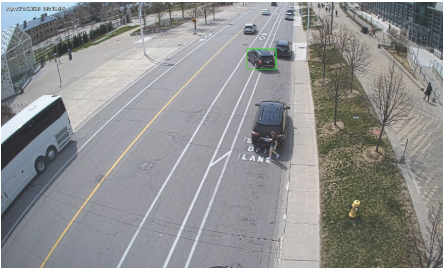
Figure 5: A full colour image taken from the Automotus platform capturing a vehicle as it departs the parking zone. This system uses AI to process high resolution video data. The data processing takes place in real time in a computer mounted to the pole, and only low-resolution images such as this one are stored and transmitted. This approach helps mitigate privacy and cybersecurity concerns.
