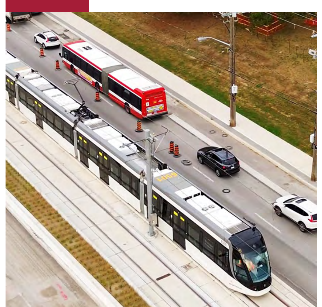
An example of an LRV from Finch West LRT. The vehicle is 48 metres long, has a seating capacity of 120 passengers and a maximum capacity of 292 passengers.
