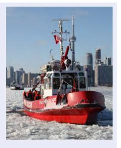
The William Thornton (WT) is a 69-foot repurposed Coast Guard Cutter that provides rapid rescue response and assists in accessing areas not passable by the larger WLM fireboat. It also serves as a backup in larger emergency situations.
