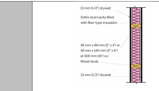
Note 1: The inclusion of fibre-type insulation (which may include glass or cellulose fibre) within the cavity of the wall assembly is provided in reference to sound absorption requirements and will provide a portion of the overall duration of the fire-resistance of the assembly.
