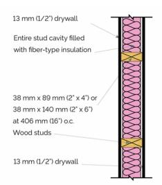
**Note 1:** The inclusion of fibre-type insulation (which may include glass or cellulose fibre) within the cavity of the wall assembly is provided in reference to sound absorption requirements and will provide a portion of the overall duration of the fire-resistance of the assembly.
