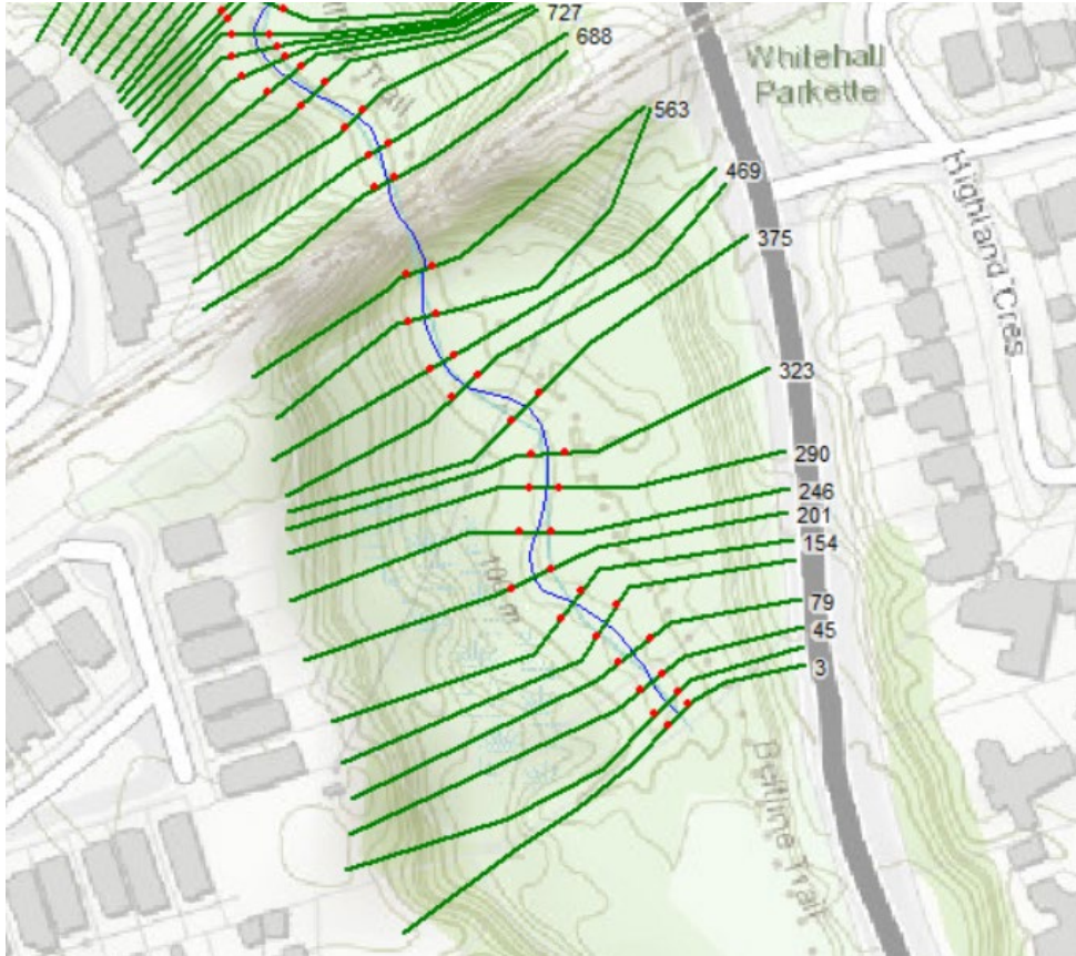
Figure 4 Location of Cross-sections throughout Reach 4 (HEC-RAS 5.0.7)
