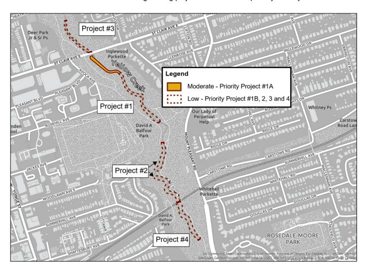
**Project 1**: The recommended solution is 340 metres of channel engineering works divided into Project #1A (85 m) and Project #1B (255 m) to reflect the higher priority need of the storm sewer outfall at the northern segment of the project area. The southern segment includes removal of concrete debris at a historic sawmill site.
