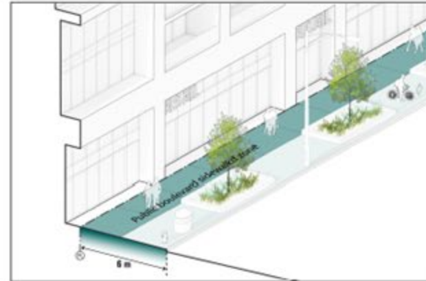
Figure 4.1.1: Illustration of commercial frontage with a generous sidewalk zone to support an active frontage and vibrant pedestrian environment.
