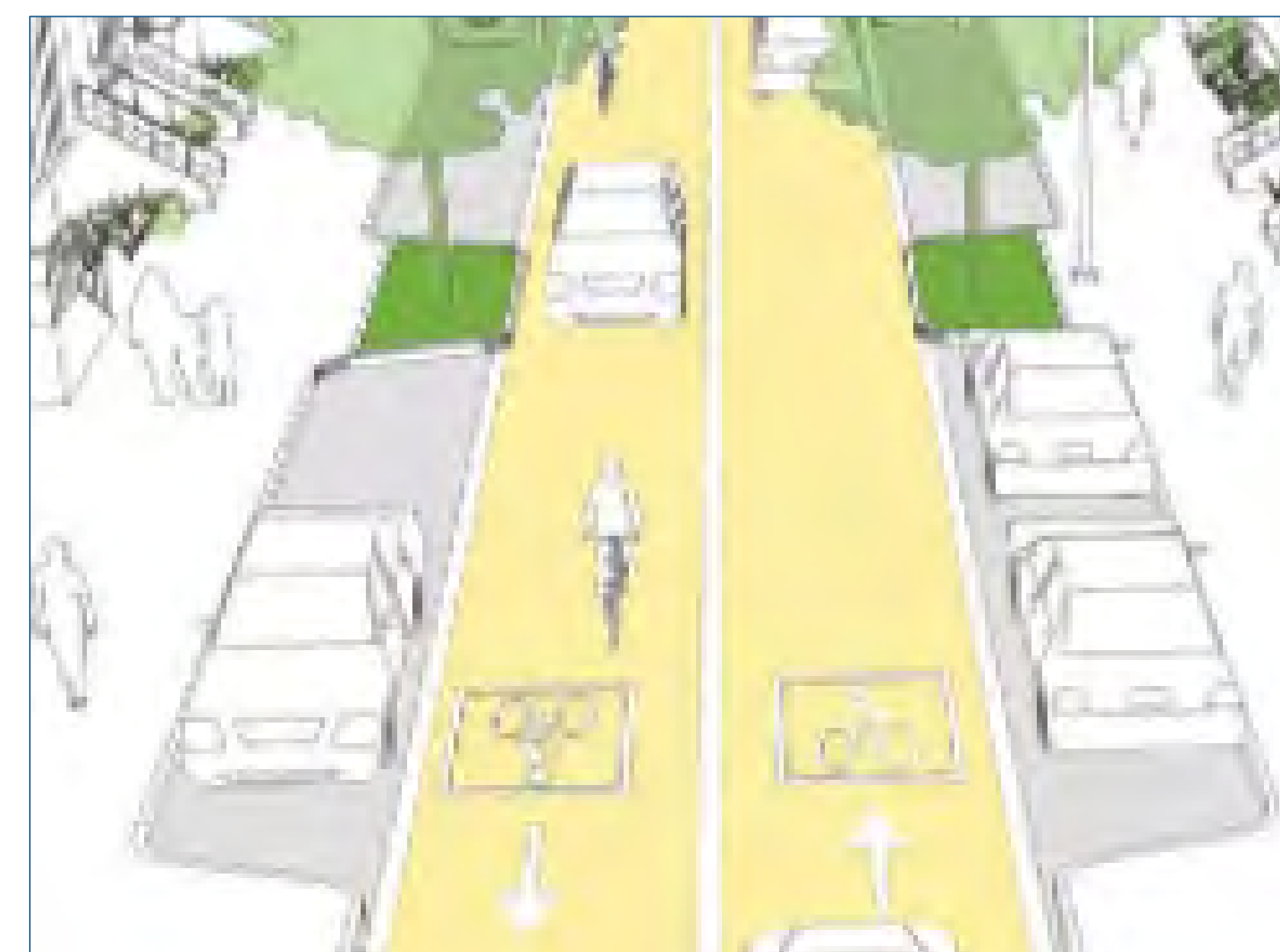
Lane narrowing or edge lines (source: NACTO)
