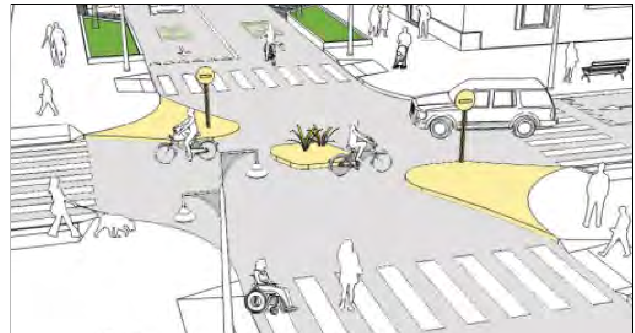
Illustration of a diagonal diverter (source: NACTO)
