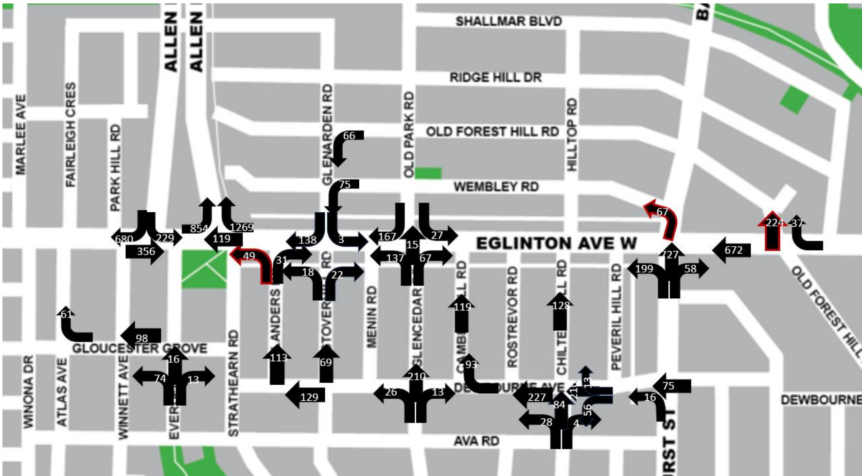
PM Peak Traffic Volumes (Feb 2025) . Arrows outlined in red = high volumes of restricted movements
