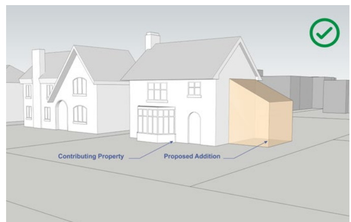
Figure 36: Contributing Property - compatible addition (view from street).
