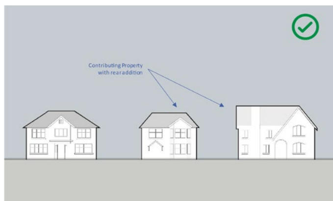
Figure 39: Contributing Property - rear additions (view from street).
