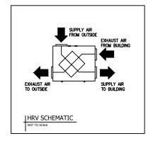
OBC 9.32.3.4.(5) AN OUTDOOR AIR SUPPLY SHALL BE INSTALLED BETWEEN THE OUTDOORS AND THE FURNACE RETURN AIR PLENUM AND SHALL BE CONNECTED (A) NOT LESS THAN 3 M UPSTREAM OF THE PLENUM CONNECTION TO THE
