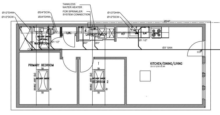
Ø3/4" C/W CONNECT TO MAIN HOUSE WATER SERVICE PIPE (OUTSIDE THE HOUSE) (WHEN SPRINKLER SYSTEM INSTALLED PROVIDE Ø2" MAIN C/W PIPE)
