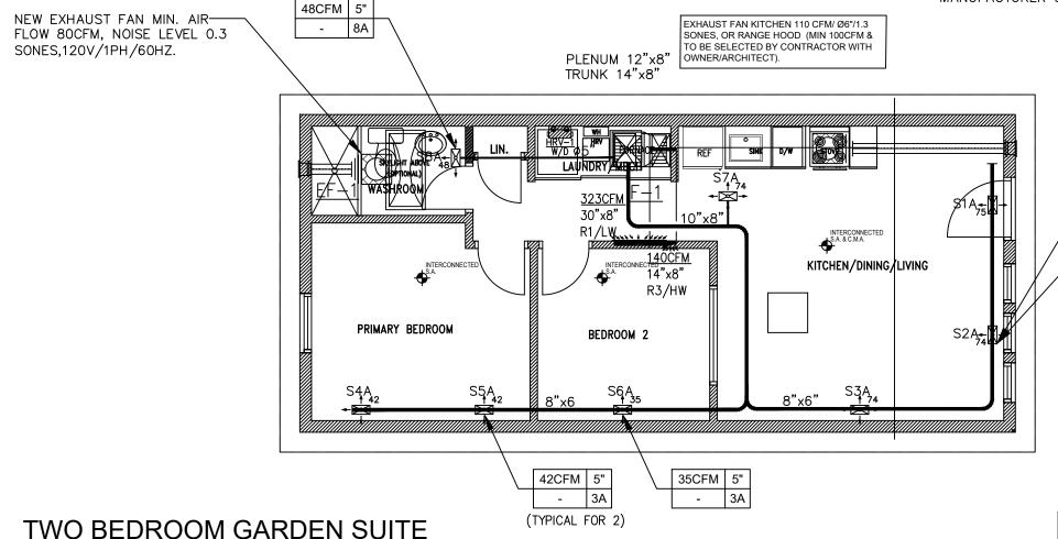
OBC 9.32.3.13.(3) THE DISTANCE SEPARATING AIR INTAKES FOR MECHANICAL VENTILATION FROM EXHAUST OUTLETS THAT ARE POTENTIAL SOURCES OF CONTAMINANTS, SUCH AS GAS VENTS OR OIL FILL PIPES, SHALL BE NOT LESS THAN 1800 mm. (REFER TO KITCHEN EXHAUST AND ERV/HRV INTAKE LOCATIONS).
