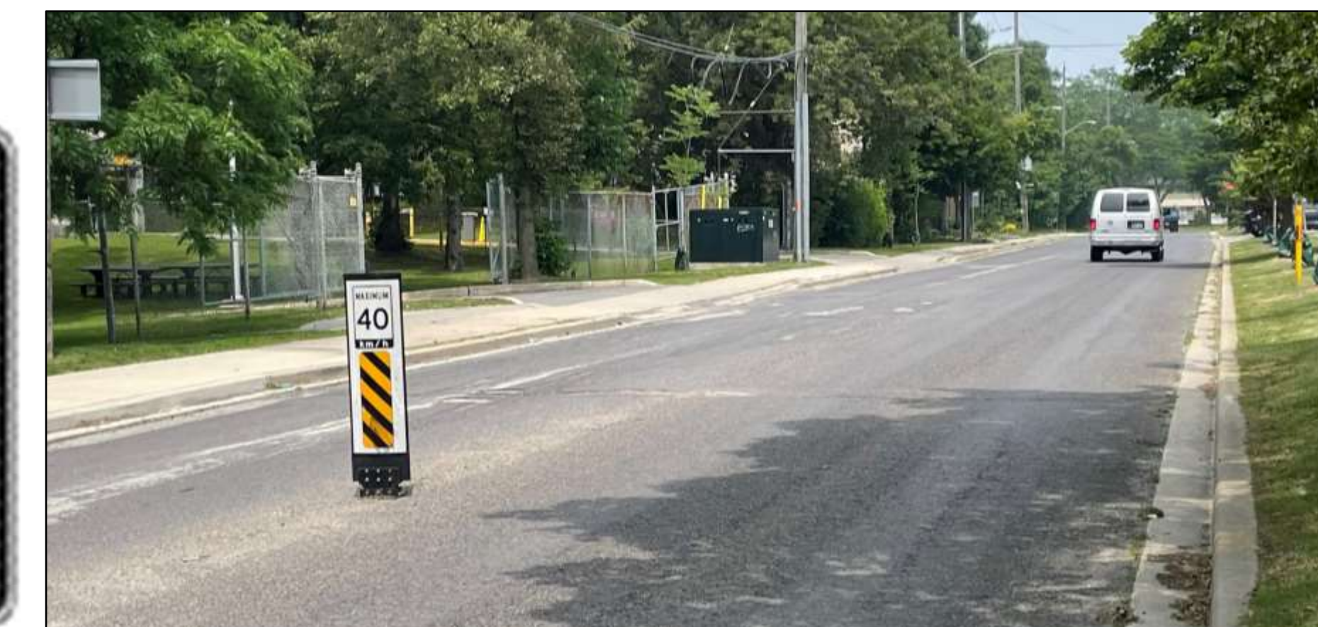
In-Road Speed Signs
