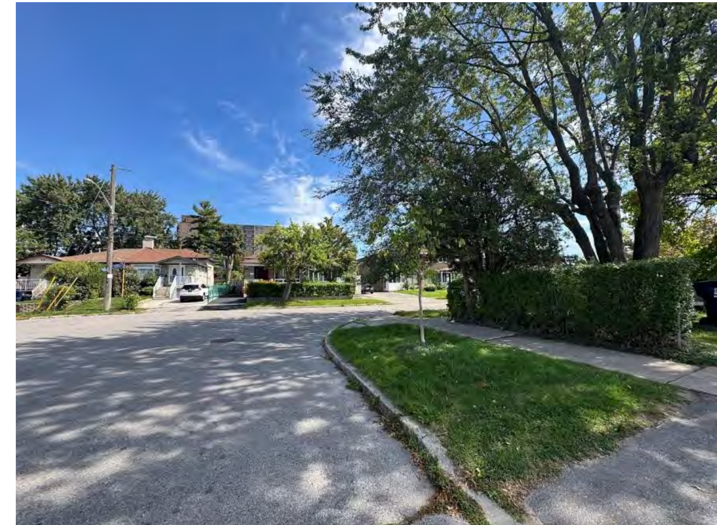
Sightline issues caused by overgrown hedges impacting visibility for turning vehicles.
