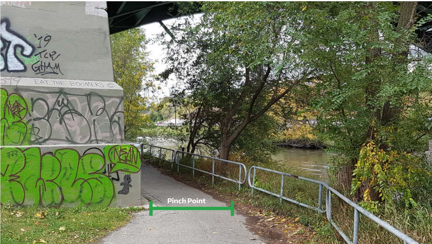
Figure 2.5 Along the Don Trail, a bridge support creates a pinch point. The multi-use trail has to be narrowed for a short distance. This is an acceptable and unavoidable reason to use a lower limit value.
