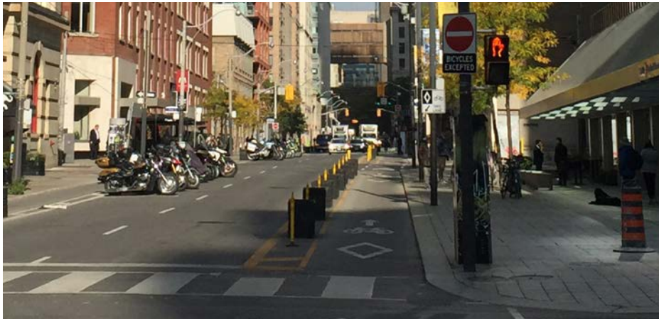
Figure 3.43 A contra-flow cycle track with flex bollard and planter separation (Option B).
