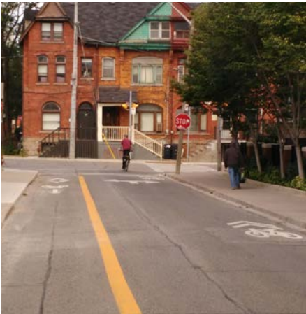
Figure 3.45 A contra-flow bicycle lane with no parking and a wide travel lane with sharrows positioned to the side. (Option A)
