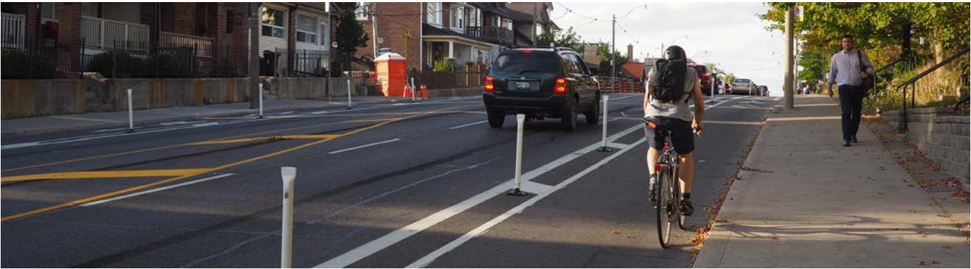
Figure 3.16 Woodbine Avenue cycle tracks, separated from the roadway by flexible bollards.
