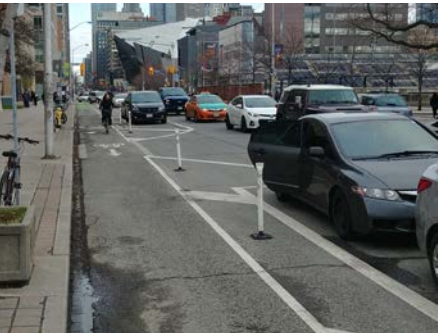
Figure 3.12 Flex bollards used as a separation technique adjacent to parking for a pilot project.
