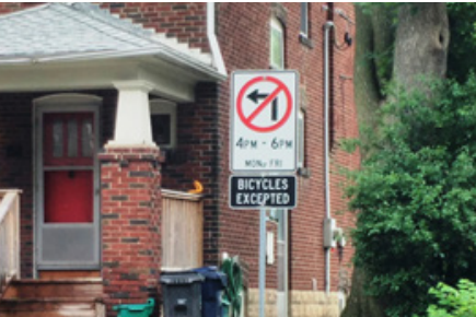
Figure 3.54 A left turn restriction with a "bicycles excepted" tab (Rb-17t).
