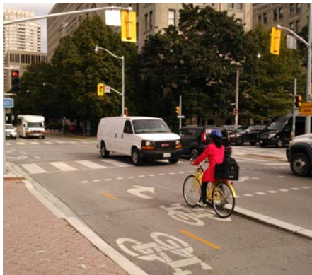
Figure 3.19 Signal and crossroad treatment for uni-directional to bi-directional transition.
