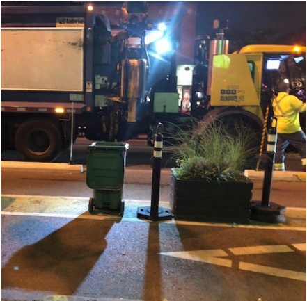
Figure 3.25 Space is left in the buffer of the Danforth cycle tracks to facilitate bins being moved from the boulevard to the collection truck
