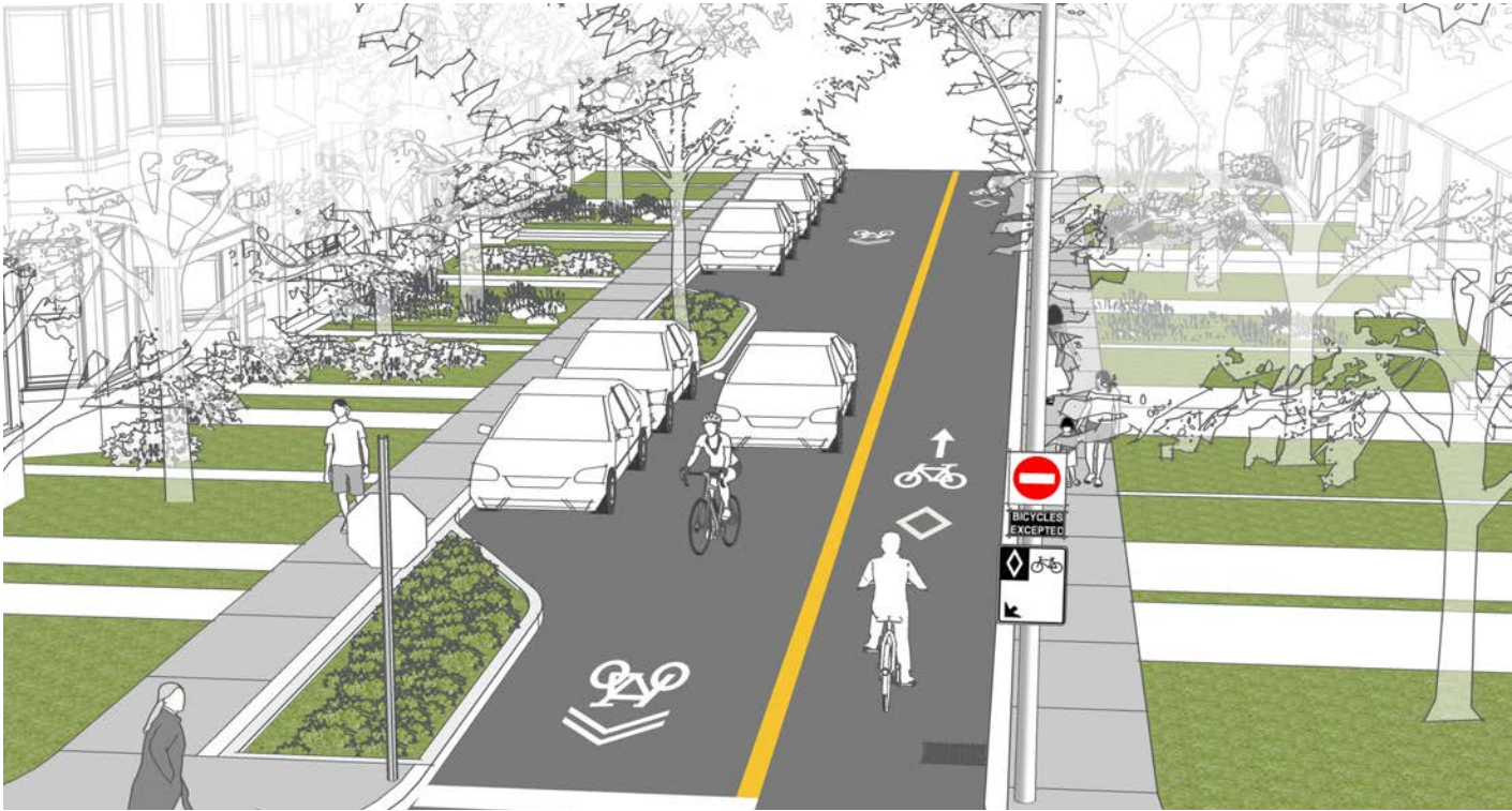
Figure 3.44 A contra-flow bicycle lane positioned between a travel lane and the curb.
