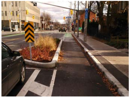
Figure 3.14 Landscaped medians can enhance aesthetics and create a transition where parking is introduced or discontinued.
