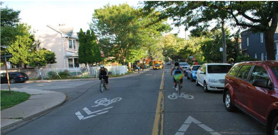
Figure 3.47 A contra-flow bicycle lane along side a parking lane and a wide travel lane with sharrows positioned to the side. This is the least preferred configuration due to parking and cycling conflicts, but can be utilized. (Option C)
