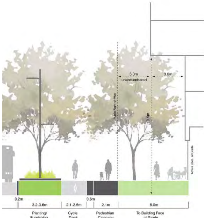
Figure 3.3 Arterial Road Setback Cross Section: Urban frontage character with commercial uses at grade
