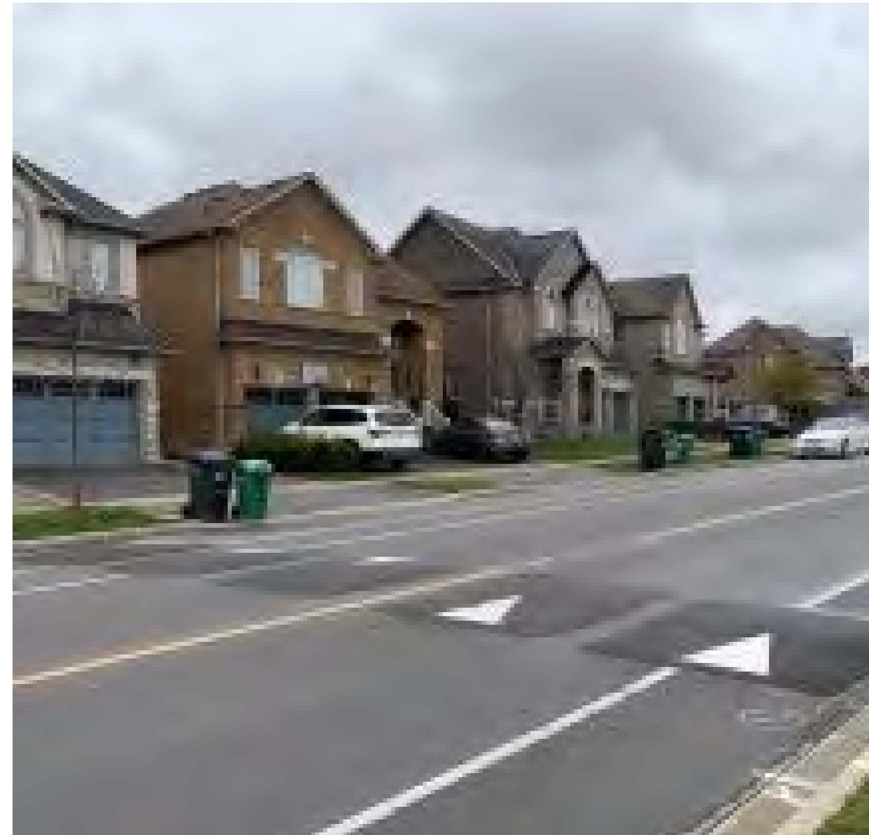
Speed cushions allow emergency vehicles to pass their wheels on either side of the raised cushion areas.
