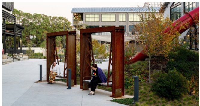
Figure 21: A real-world example of circular design in action at the Raleigh Ironworks by Future Green Studio. Old concrete from a demolished building was reused as seating blocks. Steel from an industrial structure has been repurposed into swings (Tzu Chen, 2025).
