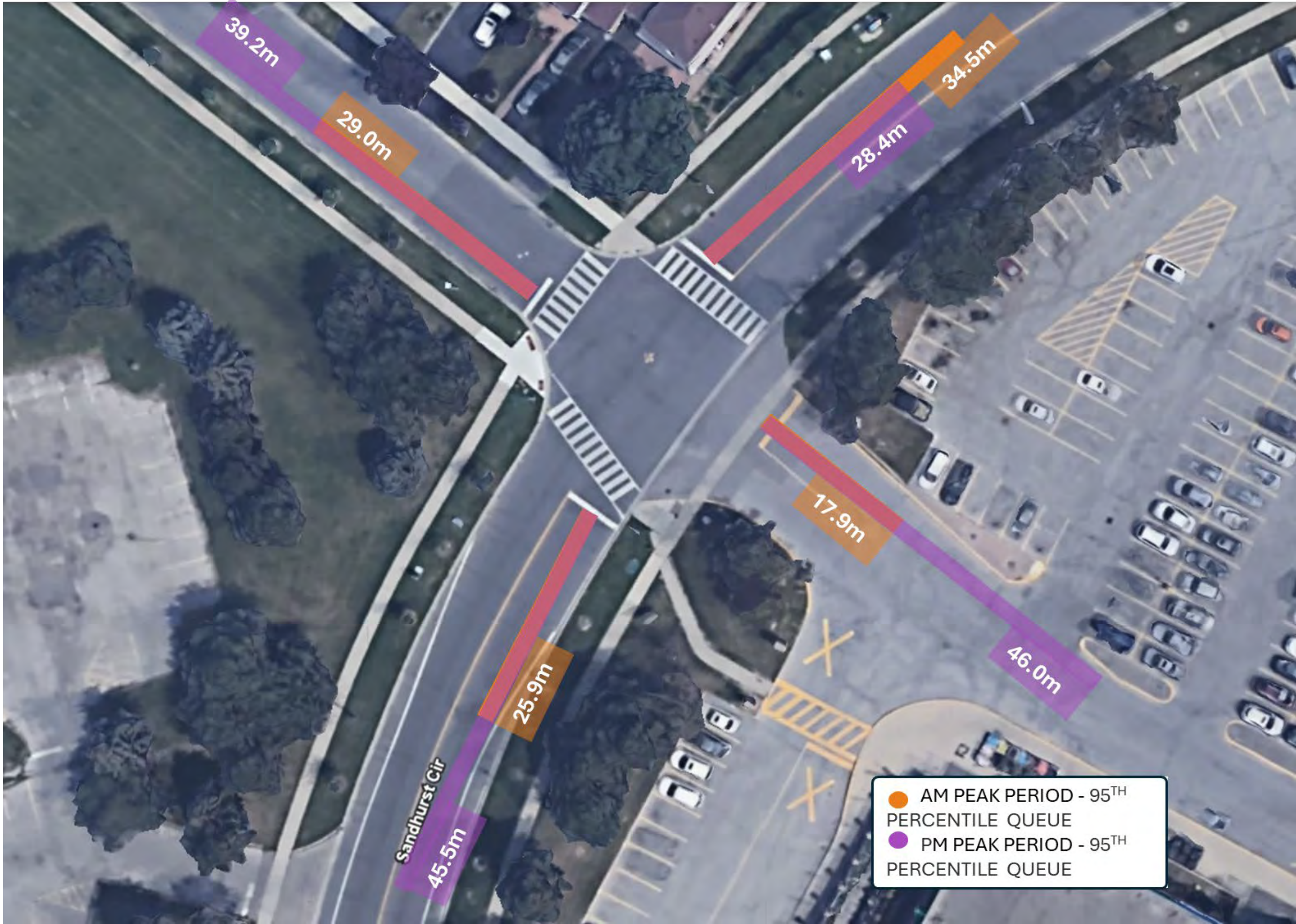
Image showing vehicle queuing during peak periods in the morning (orange) and afternoon (purple) at Sandhurst Circle and Brimwood Boulevard
