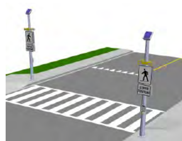
Pedestrian Crossing Signage with Flashing Lights
