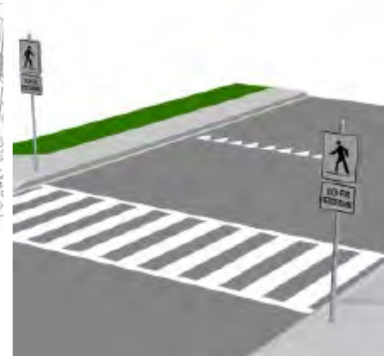
Pedestrian Crossings with Signage
