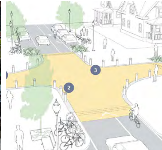
Raised Crosswalks & Intersections
