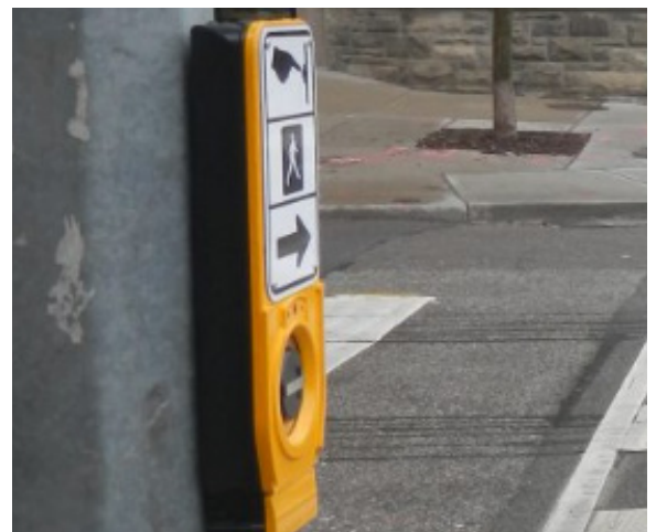
Accessible Pedestrian Signal pushbutton
