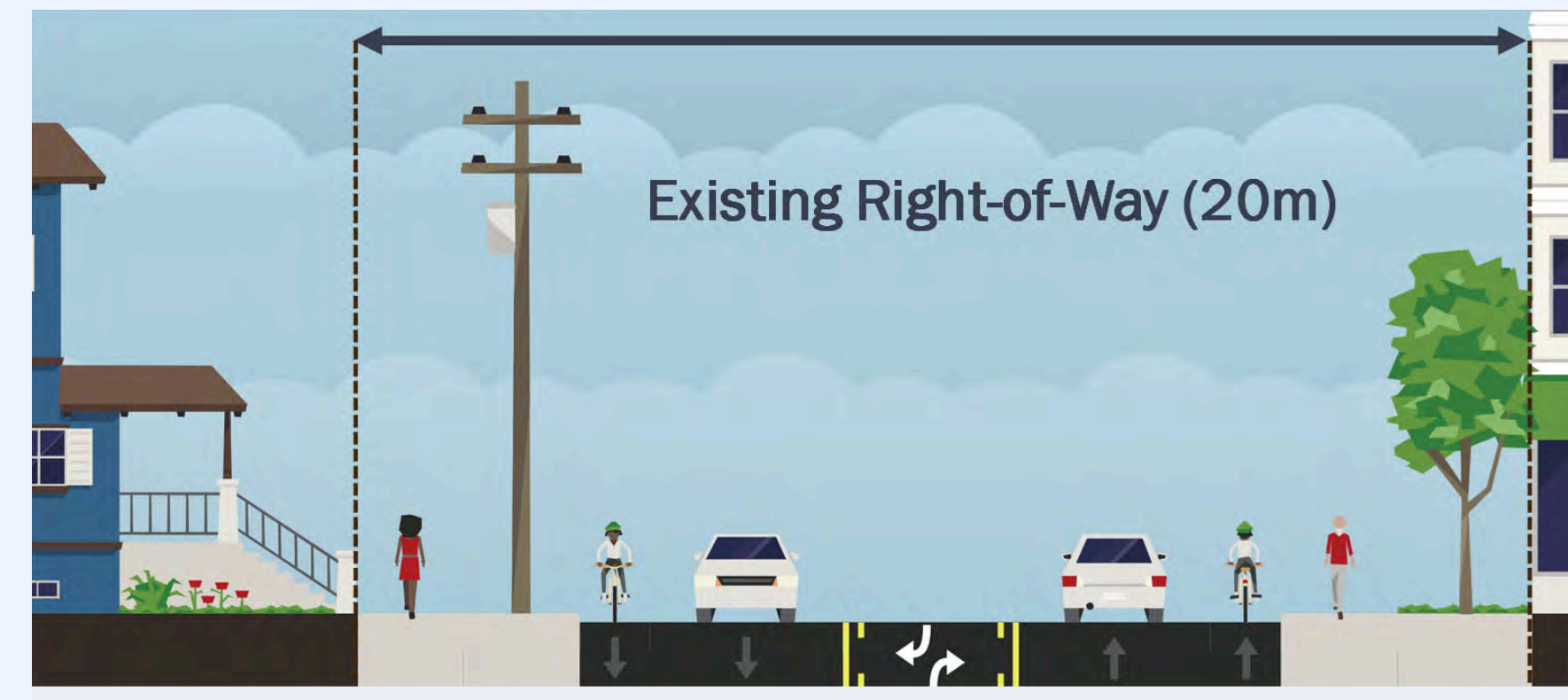
Two lanes of vehicular traffic with turning lane and bike lanes.
