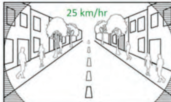
Driver's field of vision travelling at 25 km/h
