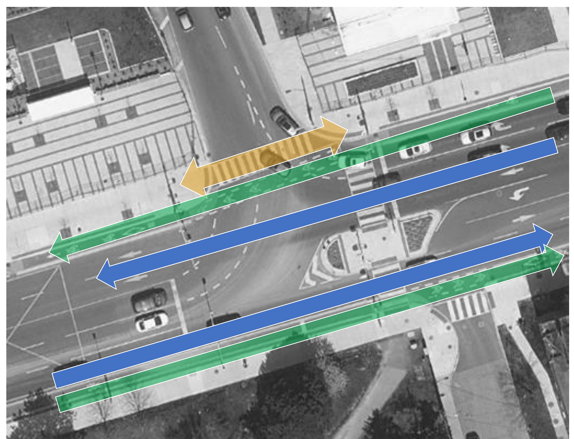
Permitted movements during the through-phase for traffic, demonstrating when pedestrians and people cycling can cross the on-ramp
