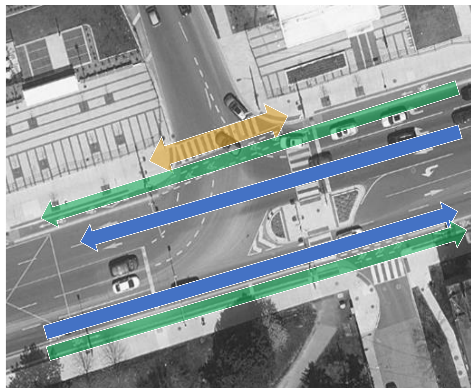
Permitted movements during the through-phase for traffic, demonstrating when pedestrians and people cycling can cross the on-ramp
