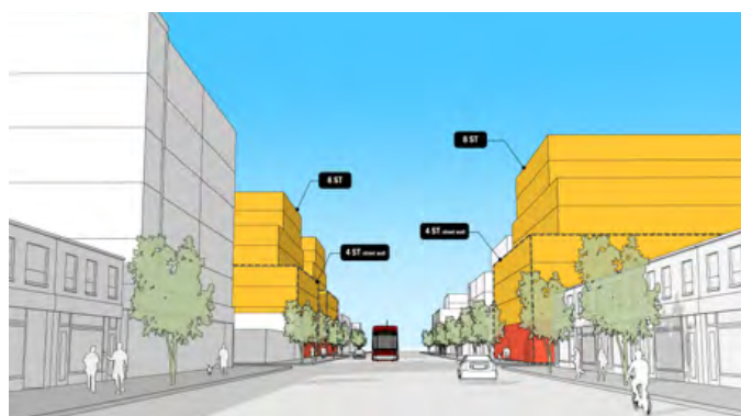
Figure 14: Street view demonstration of 8-storey mid-rise building along 27-metre right-of-ways with 4-storey streetwall height
