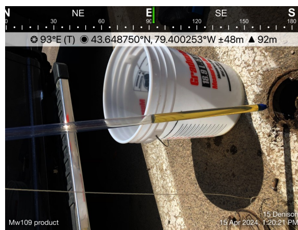
Photo 4: View of the free product layer in MW109. Photograph taken facing east.
