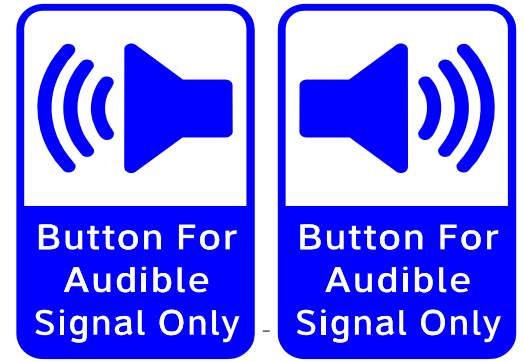
PEDESTRIAN PUSHBUTTON INFORMATION SIGN (DOUBLE SIDED BLUE SIGNS) 197mm x 127mm
