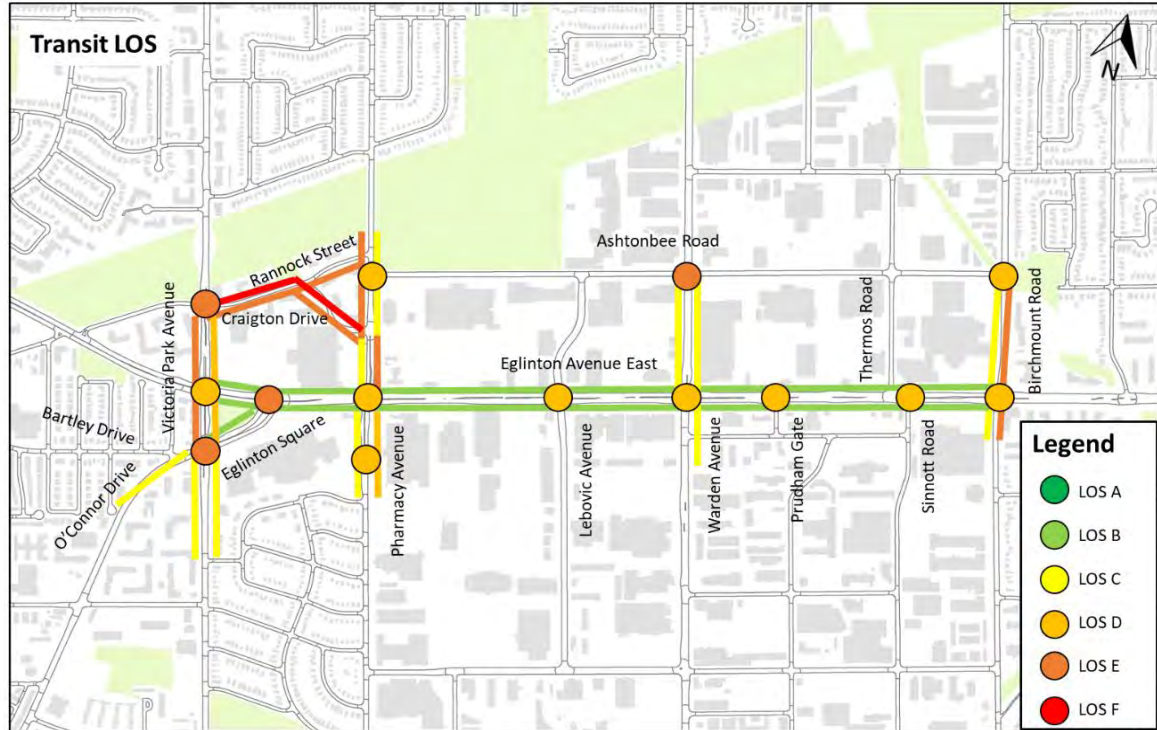
Figure 3-3: Existing (2013) Transit Level of Service Results
