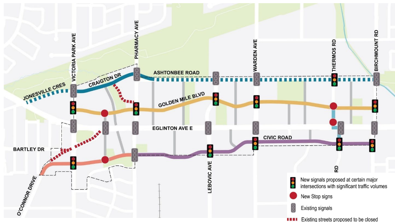
Figure 7-9: Recommended Intersection Control
